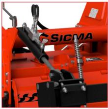
Hydraulic cylinders for roller adjustment
