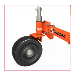
Rubber swivelling wheel to replace roller
