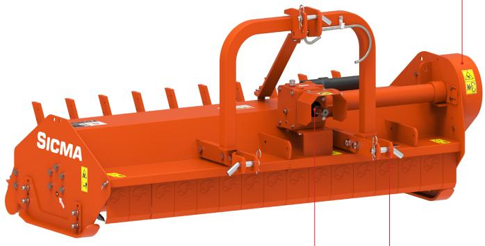
Gearbox made by SICMA, with tapered roller bearings, integrated freewheel, caps for oil input and discharge and level cap with sight glass
