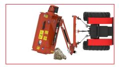
The ML Bank Mower is equipped with an anti-shock system that allows it to follow the contours of the working surfaces, protecting the structure from any damage.
