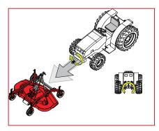
**CONFIGURATION 4.** Finishing mowers: front Rotation of tractor's PTO: **CLOCKWISE** Advancing direction: front
