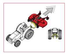
**CONFIGURATION 5.** Finishing mowers: rear Rotation of tractor's PTO: CLOCKWISE (standard) Advancing direction: rear
