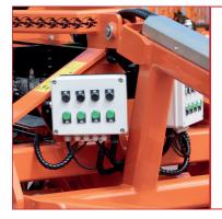
**General control panel** to adjust the working depths of the entire cultivator (available on request).
