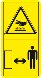
ATTENTION BURNS HAZARD
